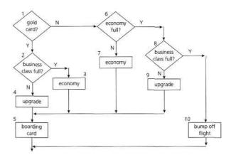
FIGURE 7.1 Control flow diagram for flight check-in
