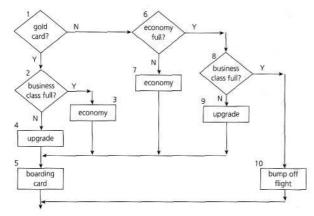
**FIGURE 4.5** Control flow diagram for flight check-in **Question 14** Why are error guessing and exploratory testing good to do?
