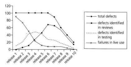
FIGURE 1.3 Changes in defect numbers during process improvement
