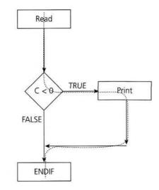
FIGURE 4.4 Control flow diagram for code sample 4.3
