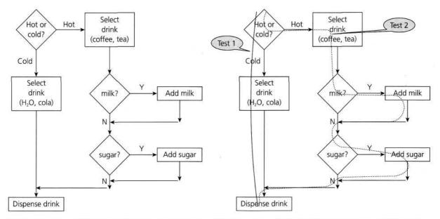
FIGURE 4.8 Control flow diagram for drinks dispenser FIGURE 4.9 Control flow diagram showing coverage of tests
