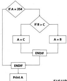
FIGURE 3.2 Control flow of a simple program
