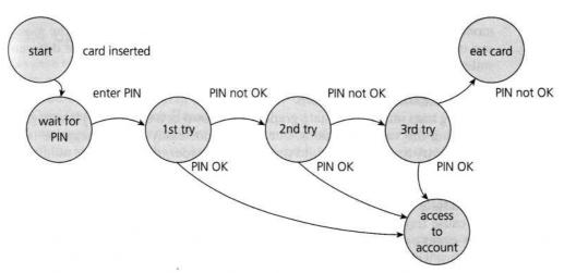
FIGURE 4.2 State diagram for PIN entry
